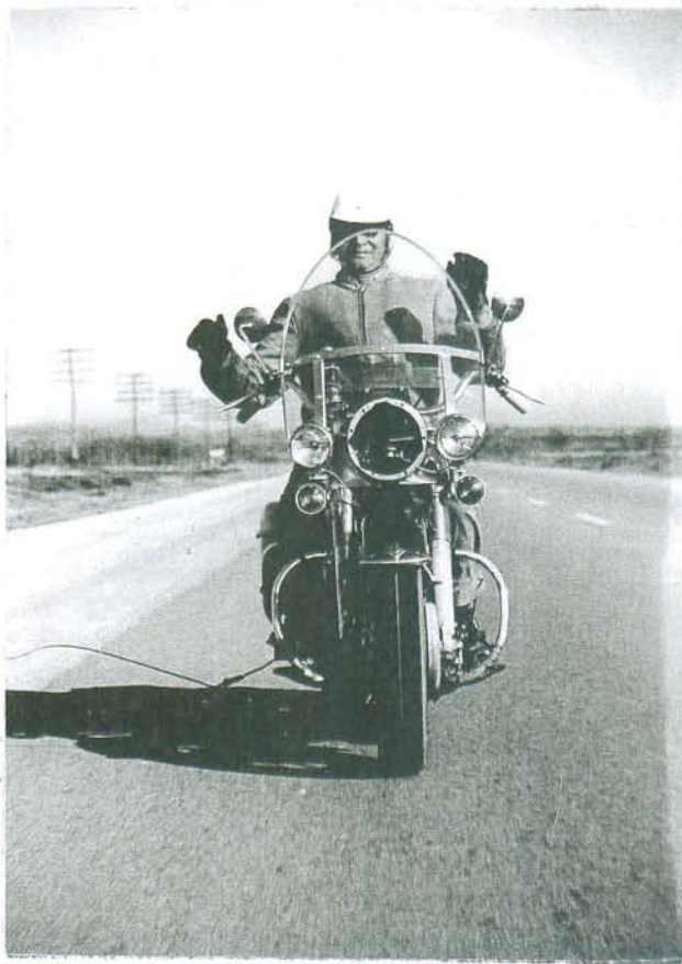
Fig. (10.9) An Actual Test Run. Driver Minimized His Input by Removing His Hands From the Handle Bar.
