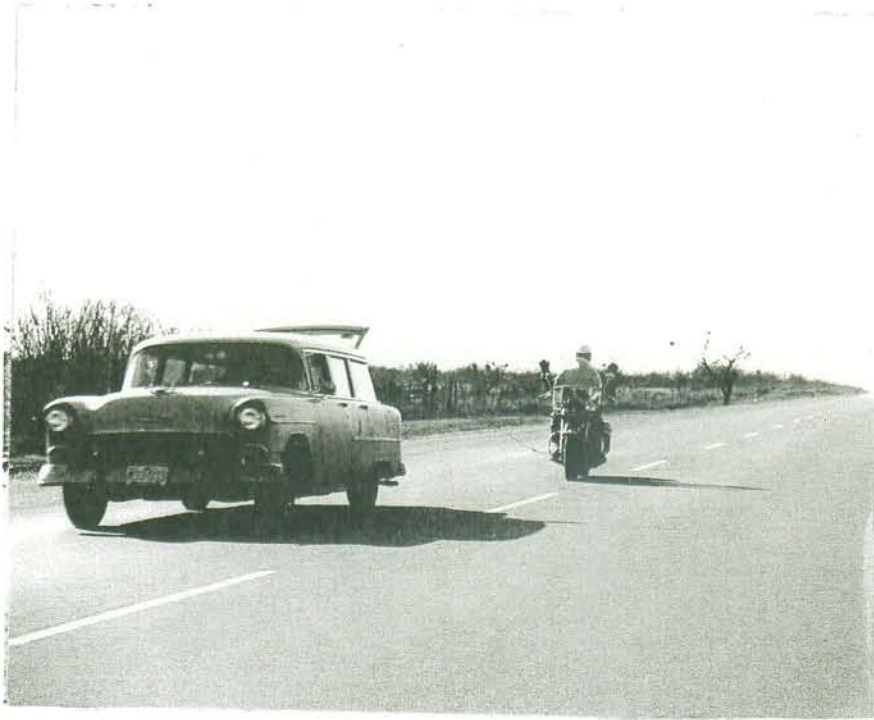
Fig. (10.7) An Actual Test Run, The Test Motorcycle Following The Slave Car Closely at the Same Speed
