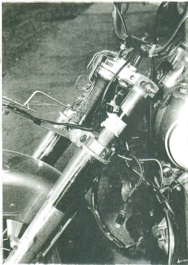
Fig. (10.2) Relocated Steering Pickup on Experimental Model with Variable Steering Geometry ( Trail Setting)
