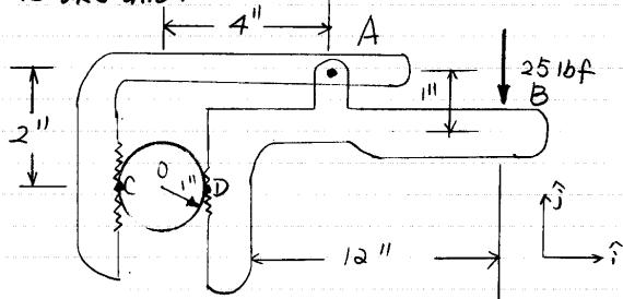
Assuming the pipe doesn't move (it's held by something), and the wrench doesn't slip, what're the forces on the pipe from wrench at C and D.
