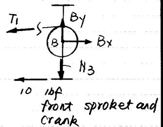
For the front chain wheel and crank:
