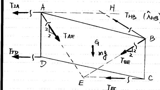
Finding  $T_{HB}$ : take the moment about axis EC: only  $T_{HB}$  and  $mg$  will produce non-zero moment about it
