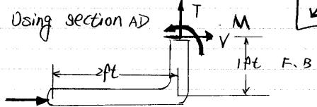
$$\begin{aligned}\sum F_x = 0 &\Rightarrow V = -RA = 6.7 \text{ lb f} \\ \sum F_y = 0 &\Rightarrow T = 0 \\ \sum M_D = 0 &\Rightarrow RA(1ft) + M = 0 \\ &\Rightarrow M = -RA \text{ ft} \\ &= -6.7 \text{ ft} \cdot \text{lb f}\end{aligned}$$
