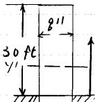
$$\begin{aligned}W &= 8gV = 8gA(30ft-y) \\ &= 8g\pi\left(\frac{9}{2} \text{ in}\right)^2(30ft-y) \\ &= 8g\pi\left(\frac{9}{2} \cdot \frac{1}{12} \text{ ft}\right)^2(30ft-y) \\ &= \pi(60 \frac{\text{lb m}}{\text{ft}^3})(\frac{1\text{bf}}{1\text{bm}})\left(\frac{81}{24^2}\right) \text{ ft}^2(30ft-y) \\ &= 8.44 \pi(30ft-y) \frac{\text{lb f}}{\text{ft}}\end{aligned}$$
