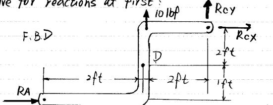
$$\begin{aligned}\sum F_x = 0 &\Rightarrow RA + RCX = 0 \\ &\Rightarrow RA = -RCX \\ \sum F_y = 0 &\Rightarrow -RCY = 10 \text{ lb f} \\ \sum M_C = 0 &\Rightarrow RA(3ft) - 10(2ft) = 0 \\ &\Rightarrow RA = 6.7 \text{ lb f} \\ &RCX = -6.7 \text{ lb f}\end{aligned}$$
