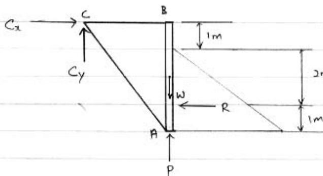
Do not leave out the reaction forces ( $C_x$  &  $C_y$ ) at the hinged joint !
