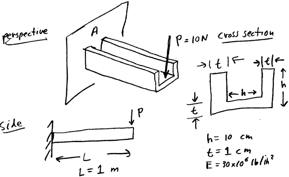
What is the ratio of the max tension stress to the max compression stress
