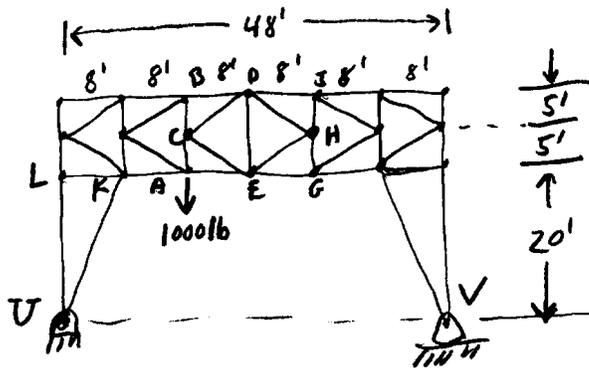
What is  $T_{KL}$  (tension in bar KL)?
