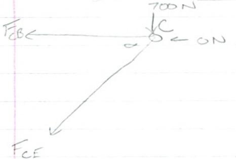
$$\begin{aligned}\sum F_x &= -F_{CB} - F_{CE} \cos \alpha = 0 \\ -F_{CB} - \frac{3}{5} F_{CE} &= 0 \\ -525 + 525 &= 0 \quad \checkmark \\ \sum F_y &= -700 - F_{CE} \sin \alpha = 0 \\ -700 - \frac{4}{5} F_{CE} &= 0 \\ -700 + 700 &= 0 \quad \checkmark\end{aligned}$$
