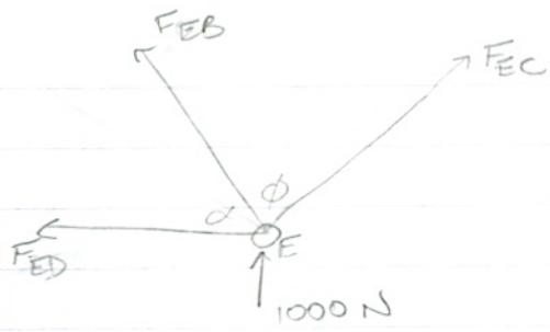
$$\begin{aligned}\sum F_y &= F_{EB} \sin \alpha + F_{EC} \sin \phi + 1000 = 0 \\ &= \frac{4}{5} F_{EB} - \frac{4}{5} F_{EC} + 1000 = 0 \\ F_{EC} &= -F_{EB} - 1250 \\ F_{EC} &= 375 - 1250 \\ F_{EC} &= -875 \text{ N}\end{aligned}$$
