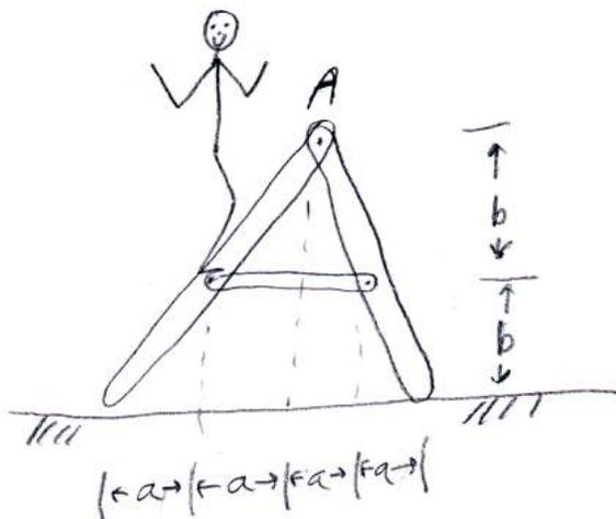
3) A massless bead slides in a rigid frictionless slot. It is held in place by the force  $F$ . Find  $F$  in terms of  $k$  and  $a$ .
