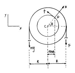
Note that the position of D is not determined yet. i.e. O is still an unknow. So in this FBD, we totally have 4 unknowns:
