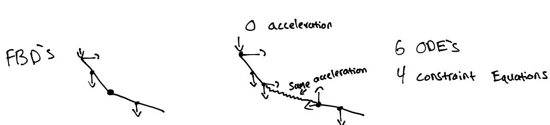
Solve for  $\ddot{\theta}_1, \ddot{\theta}_2, \ddot{x}_1, \ddot{y}_1, \ddot{x}_2, \ddot{y}_2$ , 4 constraint forces
