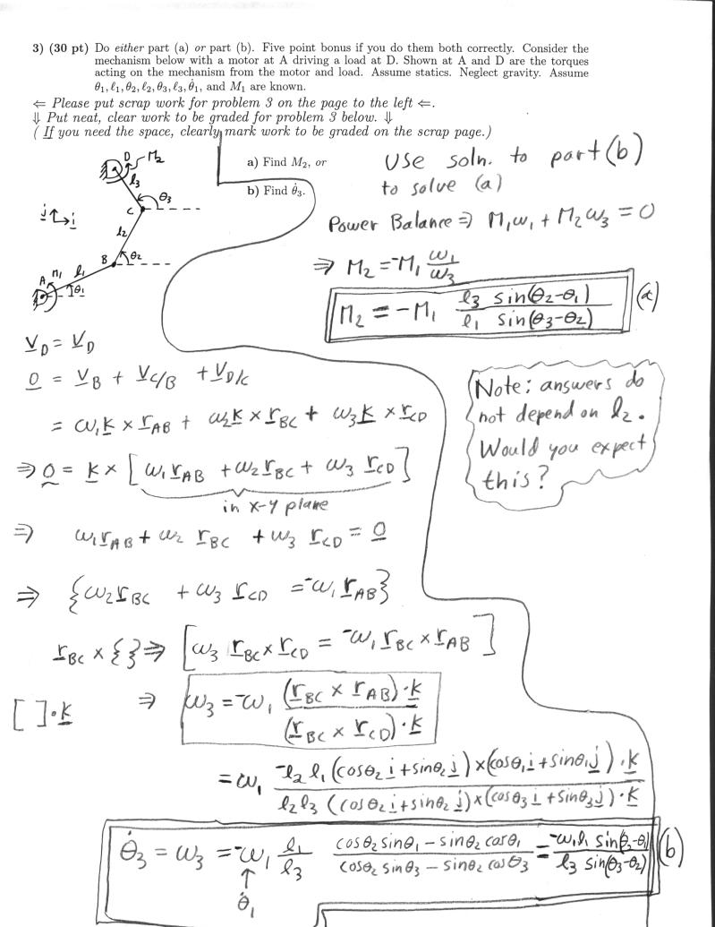
Alternate Solution to part B  $\int_{AB} = l_1(-\cos\theta_1 i - \sin\theta_2)$   $V_D = V_D$   $O = W_3 K \times C_C D + W_2 K \times V_B C + W_1 K \times V_A B$   $\{ D = (-W_3 l_3 \cos\theta_3 i + l_1 w_5 \sin\theta_3 i) + (-W_2 l_2 \cos\theta_2 i + l_3 w_2 \sin\theta_3 i) + (-W_2 l_3 \cos\theta_2 i + l_3 w_2 \sin\theta_3 i) \}$   $\{ (-W_1 l_1 \cos\theta_1 i + l_1 w_1 \sin\theta_3 i) \}$
