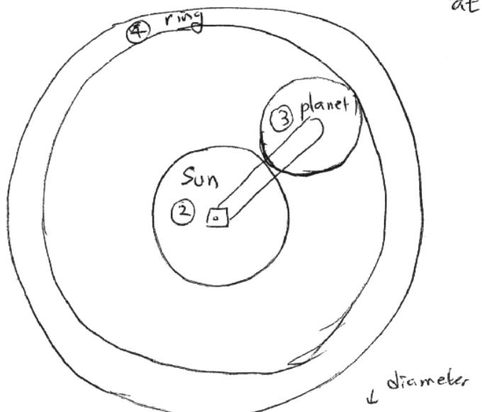
From figure,  $dr = \frac{ds}{\text{diameter of sun gear}} + 2 \frac{dp}{\text{diameter of planet gear}}$
