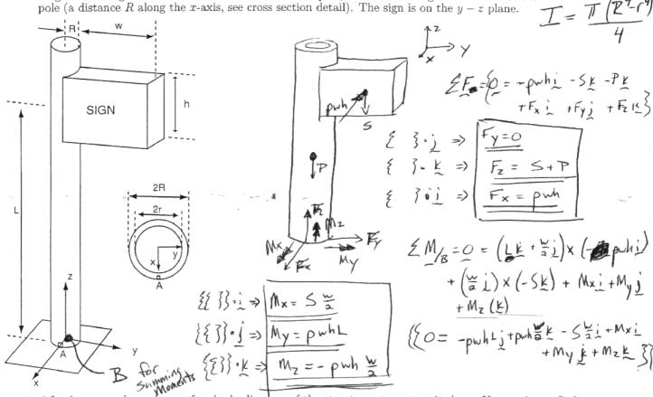
a) (10 points) In the space above draw a free-body diagram of the structure at a cut at its base. Use statics to find the forces and moments at this cut in terms of (some or all of) P, S, L, R, r, h, w and p.
