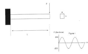
(a) Se = C<sub>10 cd</sub> C<sub>temp</sub> C<sub>reliab</sub> C<sub>Suf</sub> Se' (\$\frac{1}{5F}\$) \\
