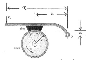
Braking Torque = Moment on drum due to friction  $M_B = Fr$ AMB/o of brake arm (Statios)  $EM_{10} = Q = (-F_a a - F_c + Nb) E$   $\Rightarrow F_a a = -F_c + F_b$   $= F(\frac{b}{\mu} - c) \Rightarrow F = \frac{F_a a}{b/\mu - c}$
