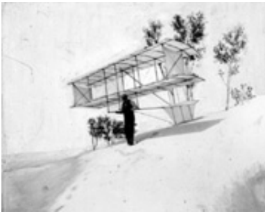
Figure 6.3: Chanute Glider, 1896. The Wright brothers' first planes were near copies of the 4-wing gliders built a few years earlier by Octave Chanute. Chanute was a retired bridge designer. Structurally these early biplanes were essentially flying bridges. The Wright brothers were preoccupied with trusses. Their first inspiration and main airplane patent was about how to control the distortion of a truss ('wing warping'). The Wrights even thought of the threads in their wing fabric as bars in a truss. Take away the outer skin from many small modern planes and you will also find trusses. (National Air and Space Museum Negative 1A-2036084-10697)
