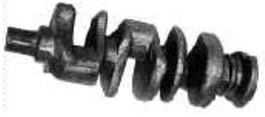
Figure 20.1: A car crankshaft is a complex three-dimensional object which is well approximated for many purposes as rotating about a fixed axis. The relative timing of the reciprocating pistons is controlled by this complex shape. “Connecting rods” are pinned to the cylinders at one end and to the short offset cylinders on the crankshaft at the other.
