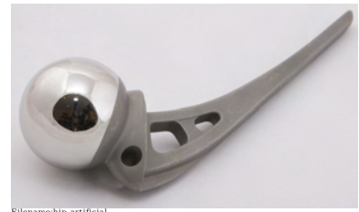
Figure 3.13: The ball part of an artificial hip joint. (Photo courtesy of Daniel Rutter, www.dansdata.com).
