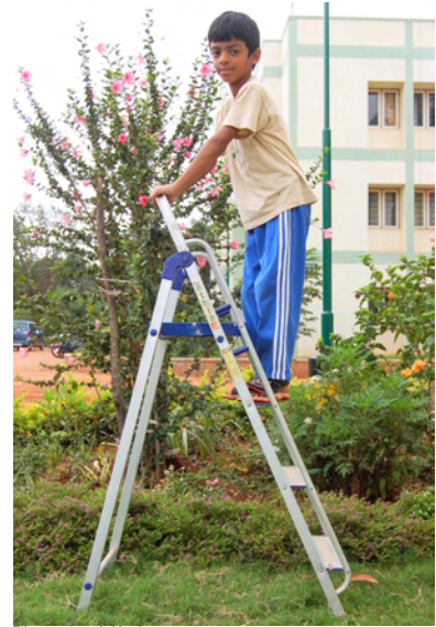
Figure 5.51: A ladder is well modeled as a collection of rigid pieces connected by pin joints ...
