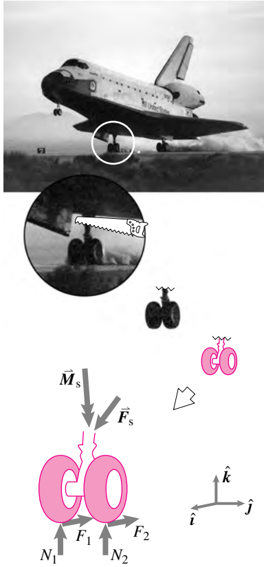
Figure 2.38: The process of drawing a FBD is illustrated by the sequence shown.
