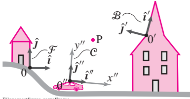
Figure 18.21: A third reference frame \mathcal{C} is defined by an origin O'' and coordinate axes x''y''z'' or base vectors \hat{i}''\hat{j}''\hat{k}'' . In this case \mathcal{C} is moving and rotating with respect to \mathcal{F} and \mathcal{B} . Once the x''y'' (or \hat{i}''\hat{j}'' ) directions are chosen the z'' (or \hat{k}'' ) direction is implicitly defined by the right hand rule.
