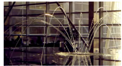
Figure 12.4: The water runs in continuous streams. Some fancy valve work (under the visible part of the fountain) is required to get such a laminar stream that holds together for the whole flight. This water draws its own graph of the trajectory of its particles. You can do the same kind of thing with a squirt gun next to a blackboard.
