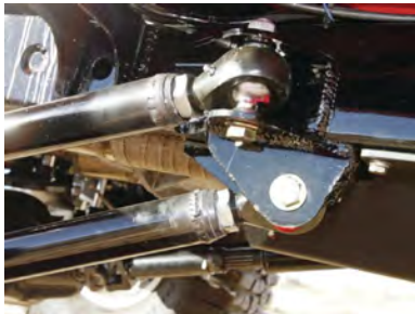
Figure 2.49: A rod end . Shown here in a jeep. A steel sphere slides in a truncated spherical cavity encased in the ‘rod end’. Often the cavity is brass encased in a the steel rod end. In this case, a lubrication grease-fitting nipple is also visible. (From fourwheeler.com)
